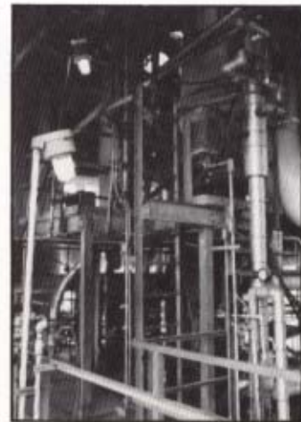
Model 794 hydraulic power/control unit and model 764 actuators in operation.
